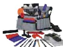
Contiene: 1 borsa porta accessori grande, 2 magneti neri, 1 daily cutter, 1 grip cutter, 1 lift stick, 1 guanti sensation, 10 felt stripes, 1 guanti bianchi, 1 paio di pinzette, 1 spatola morbida in plastica, 1 spatola dura in plastica, 1 penna forabolle, 1 raschietto, 1 solid cutter, 1 loop cutter, 1 snappy cutter, 1 design cutter.
